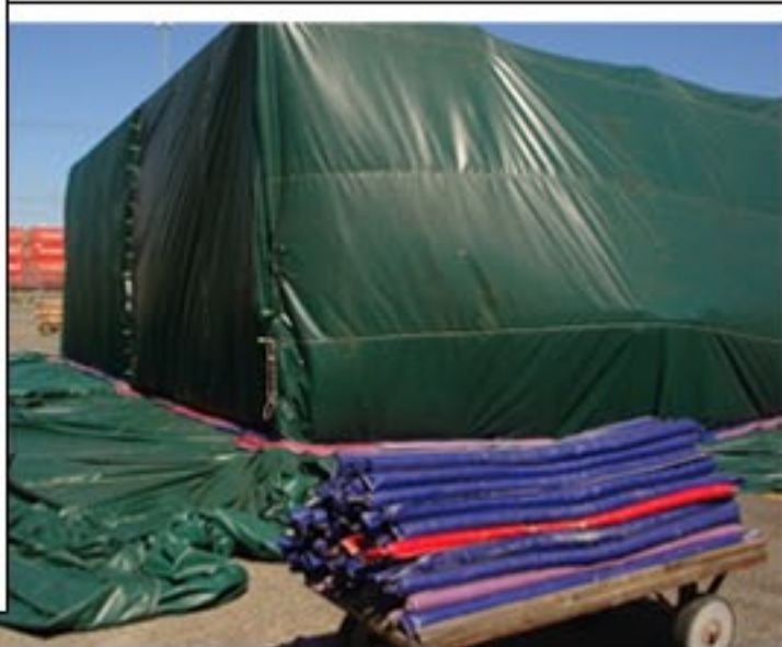
Containers under fumigation covered with nylon tarps and held tight with clips and sand snakes - Port of Tacoma
